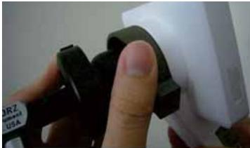
Step 4: Rotate and fasten Horus Scope Adapter in a counter-clockwise direction, where as the “switch” is at the bottom.
