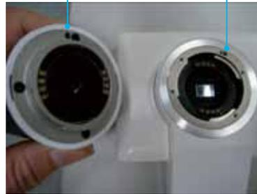
Step 2: Hold Optical Lens and attach it on Control Unit.
