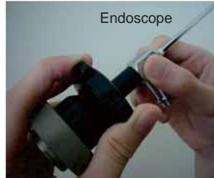
Step 2: Align the Marks of Horus Scope Adapter and Control Unit.
