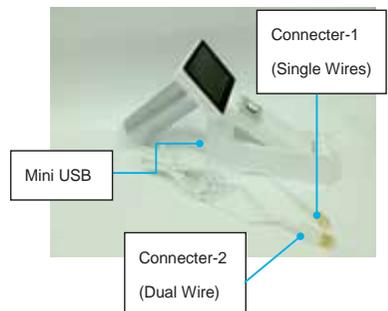
Note: Suggest charging the battery after turning off the device. If charging the battery when device is on, over charge protection design will be activated automatically after 5 hours. And then the battery will discharge until no power.
