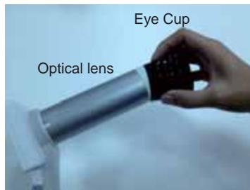
Step 2: If you want to change the direction of mask wing, one hand holds the lens, the other hand rotates mask to the direction you wanted. The idea is using the mask wing to fit the eye socket.
