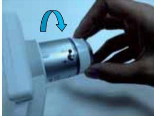
Step 2: Separate the white plastic parts, and use new one for replacement.
