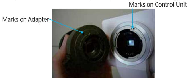
Step 3: Hold Horus Scope Adapter and attach it on Control Unit.
